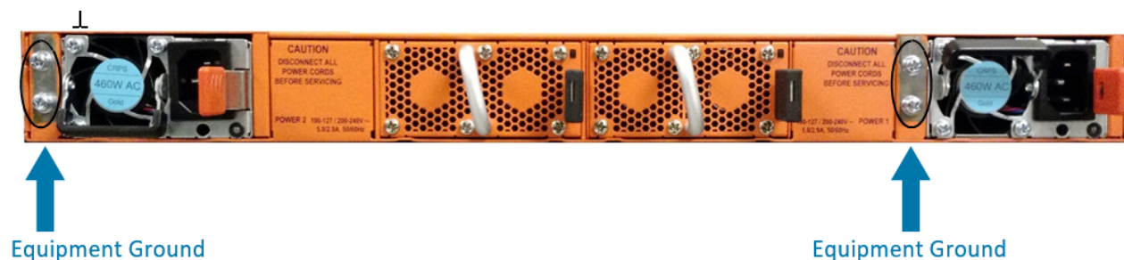
Figure 5 Ground Screws (GigaVUE TA Series Shown)
